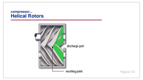
Continued rotation of the rotors causes the meshing point to travel toward the discharge end of the compressor, driving the trapped refrigerant vapor ahead of it. This action progressively reduces the volume of the pockets, compressing the refrigerant.
